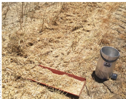
The Bushel Plus Multi Calibration System drop tray in a canola windrow with the fan-driven separator.
