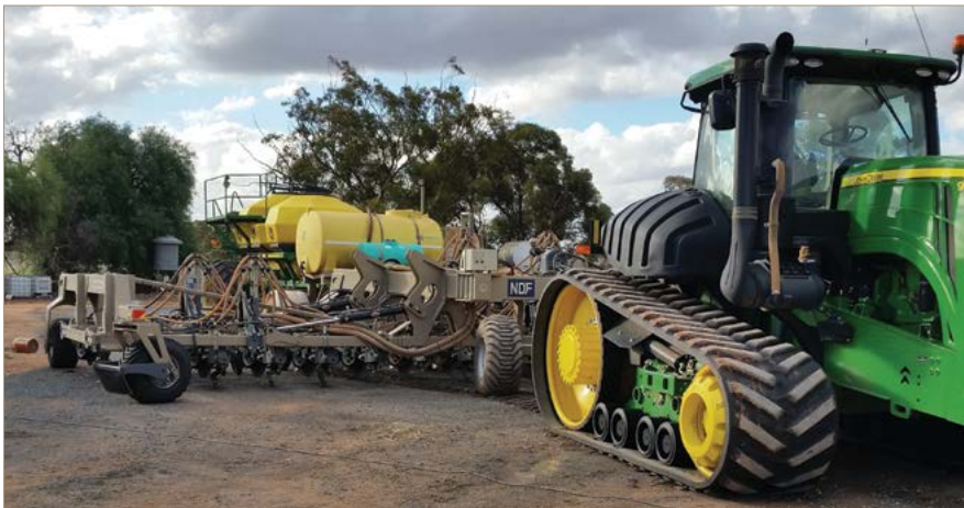
Tracked tractor and aligned 40ft (12.2m) NDF disc seeder.
