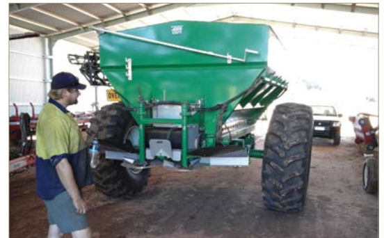
Spreader adjusted to 3m wheel spacing.
