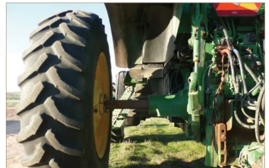
Rear axle adjustment on spray tractor.
