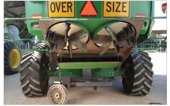
Integrated weed destructor on header.
