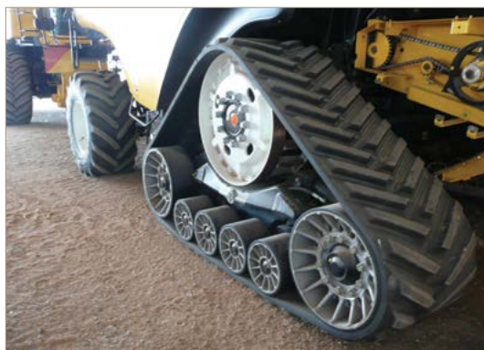
Front tracks on header.
