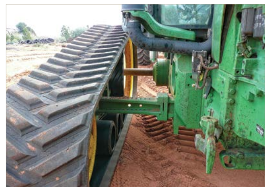
Extension adaption for 3m wide tracked tractor.
