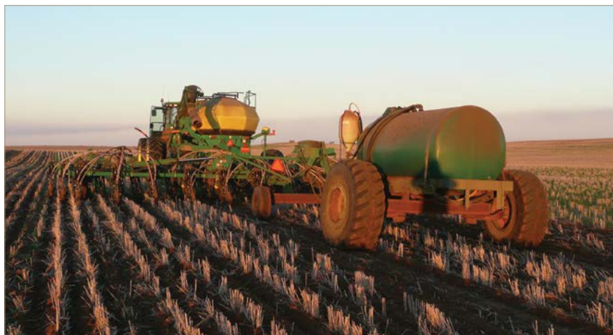
Seeding system with trailing fluid cart.
