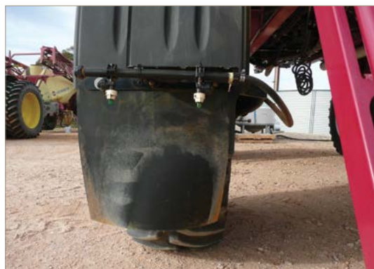
Extra spray nozzles on SP sprayer target weeds on wheeltracks.
