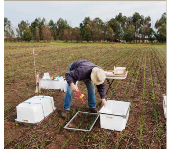
The results discussed in this report come from measuring nitrous oxide N_2O emissions from wheeltracks and untrafficked soil. It is impracticable to measure the N_2 directly, because it is already at 70 per cent of the atmosphere, whereas there is no N_2O except from the denitrification process.
