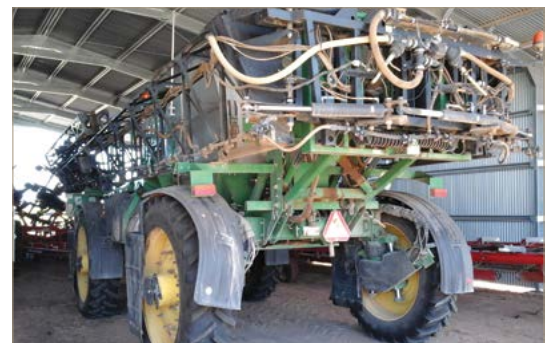
36m SP sprayer is on 3m wheel spacing.
