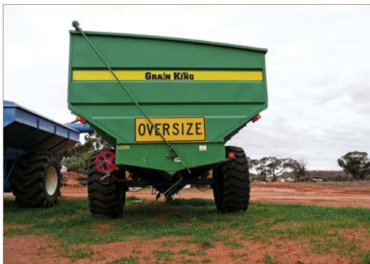
Chaser bin on 3m wheeltracks.
