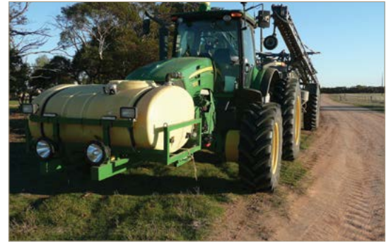
Front axle cotton reels on spray tractor.
