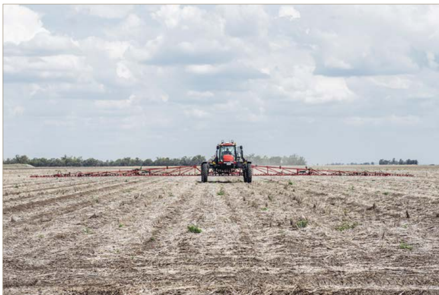
Operating machinery on firm CTF wheeltracks reduces power requirements and fuel use.
