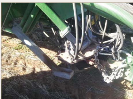
Protrakker implement guidance on the seeder.
