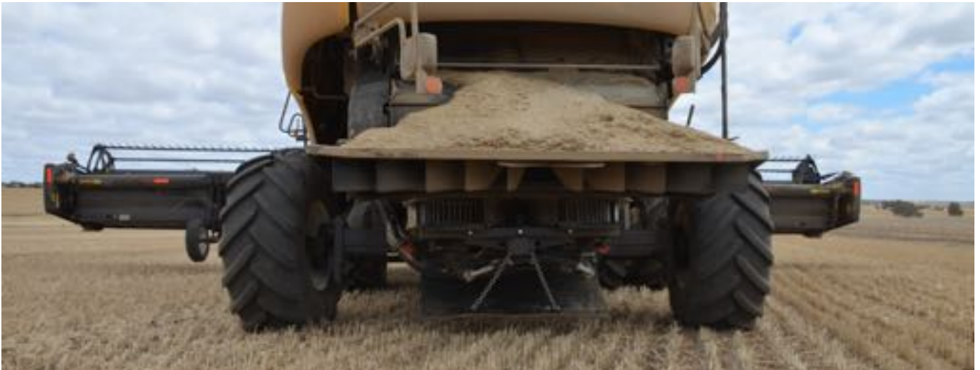
The integrated Harrington Seed Destructor
