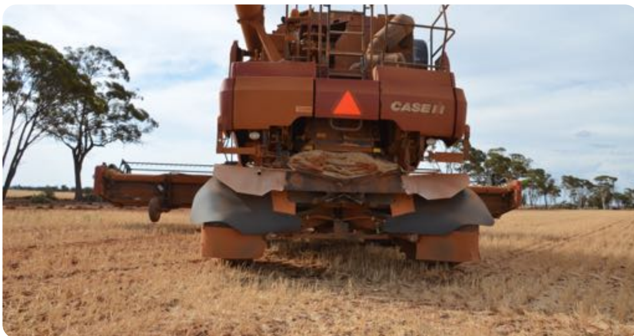
The Emar chaff deck fitted to the back of Clint's header
