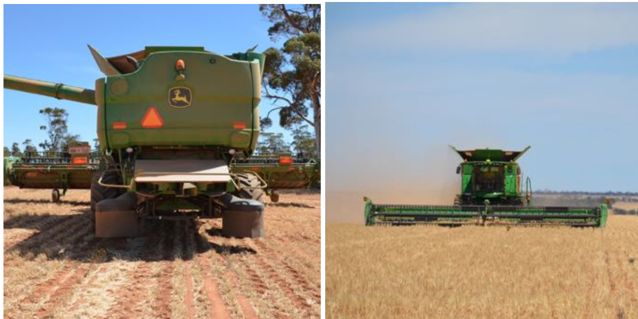
IMAGES: (L) The chaff deck (R) Harvesting at Kirby's in Beacon, note the coreflute on the header front.
