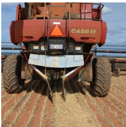
The windrow chute with the narrow windrow formed.
