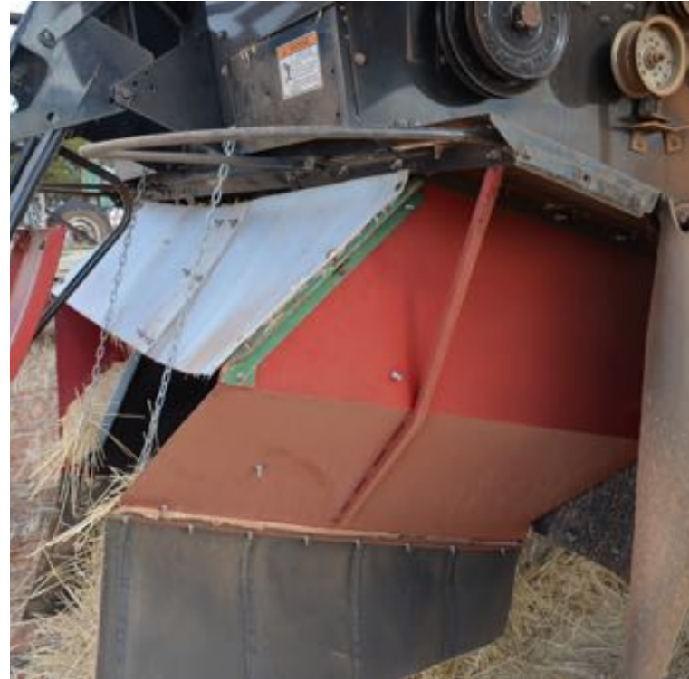
Modifications made to the windrow ensure that as much weed seed as possible is collected and deposited in the narrow windrow
