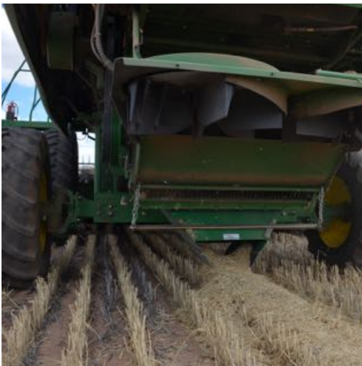
Chaff formed one line and the straw fraction is spread with this form of HWSC.
