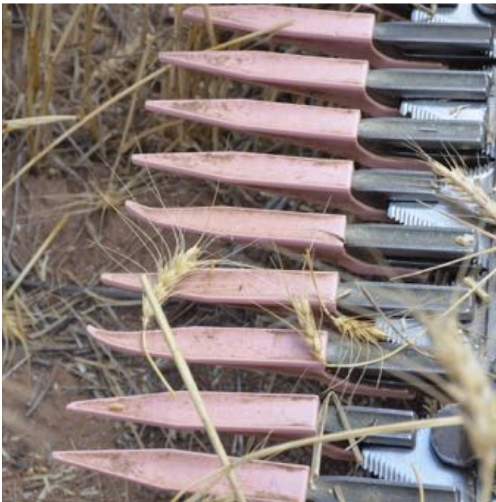
Extended fingers help to pick up more grain and weed seed in the header front .
