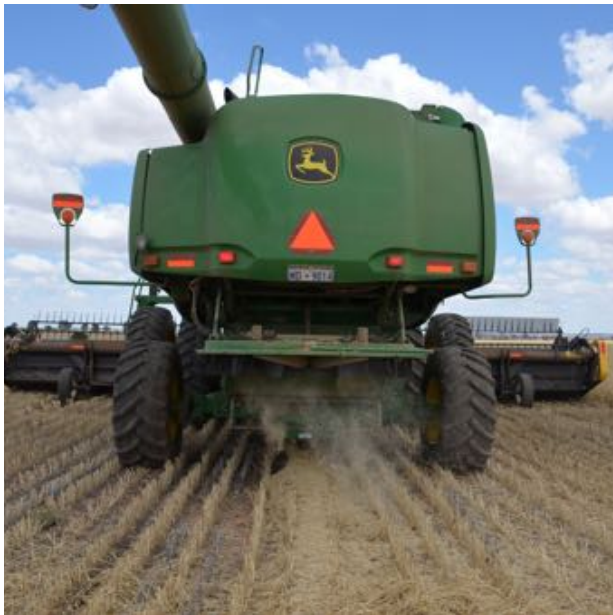
The chaff line fitted to the back of the header
