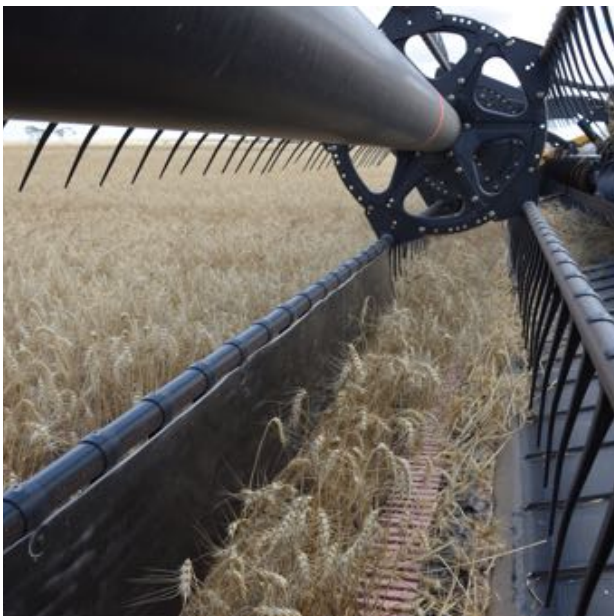
Corflute, extended fingers and a narrow knife guard fitted to the header front
