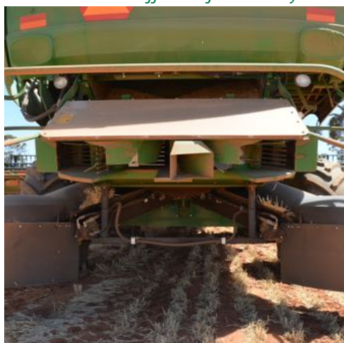
IMAGE The Emar Chaff deck fitted to Ty's header.
