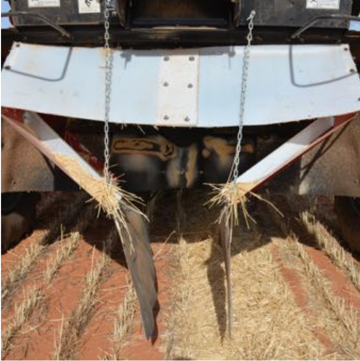
A close up of the windrow chute
