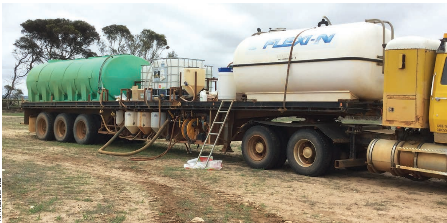
A simple tanker and batching set-up for servicing spraying operations on multiple farms.
