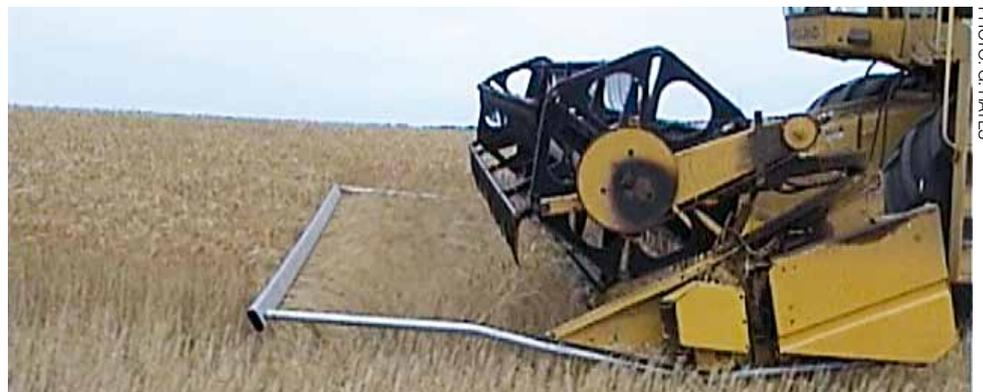
**Figure 2** A rigid pusher bar suited to cereal crops. Currently, the preferred material is 100 to 125mm DuraGal® tubing. The bar is set 2 to 2.2m in front of the knife and the lower edge is 50 to 70mm above the cutting height.
