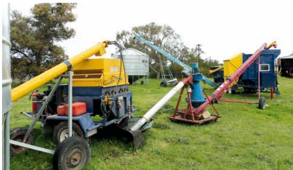
*Vigilant cleaning of harvesters and equipment will help reduce snail occurrences in future crops. Pictured here are a snail crushing roller, followed by an aspirator and a screen cleaner.*
